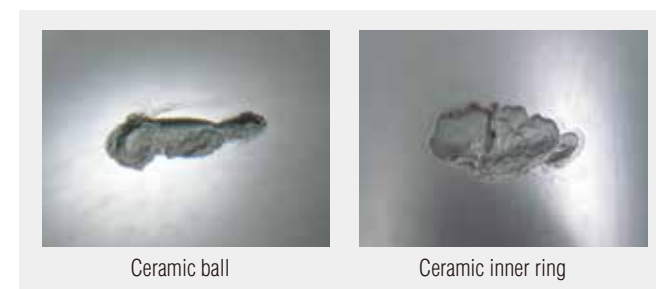
Fig. 6 Flaking on ceramic ball and inner ring
